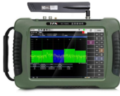
Fig. 5 The omnidirectional antenna connection of the monitoring receiver
