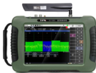
Figure 8.16 Schematic diagram of omnidirectional antenna and RMT series spectrometer
